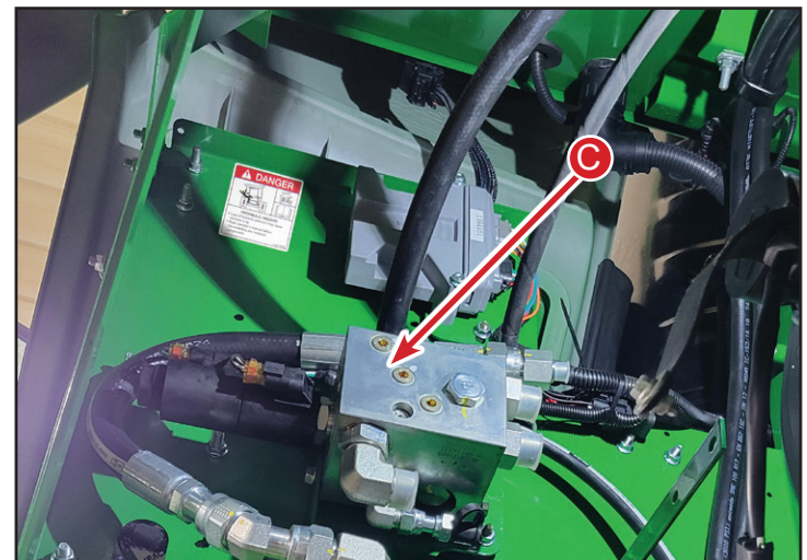
C - Leveling Manifold
