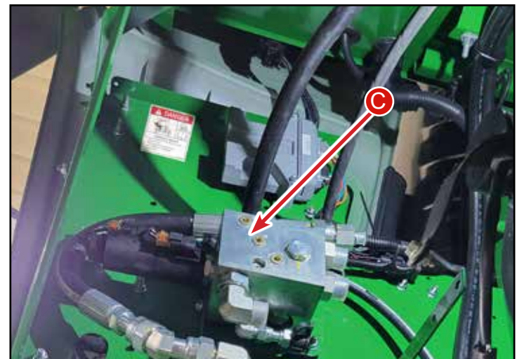
C - Leveling Manifold
