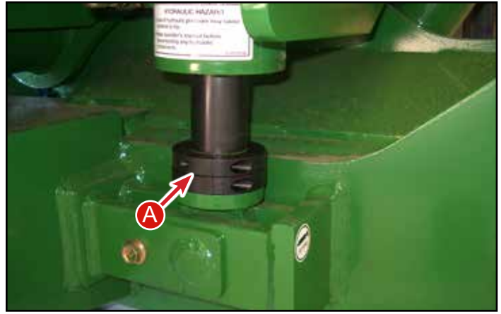
A - Mechanical Leveling Cylinder Stops 5/8 inch - Part # MC-137251 1/8 inch - Part # MC-137501
