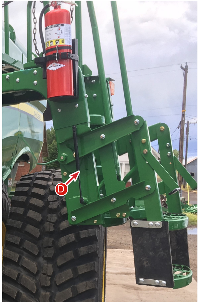
D - Gas-charged Struts
