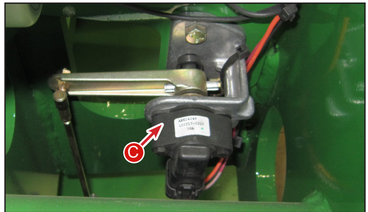
C - Undercarriage Position Indicator
