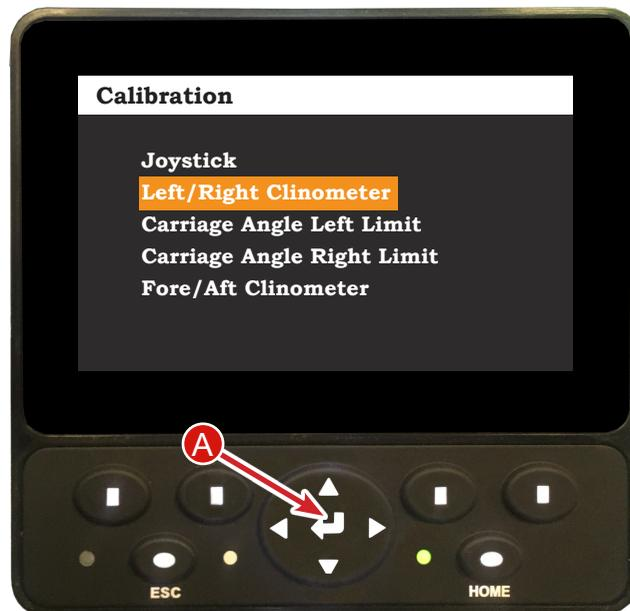
Follow the directions on the screen. When the combine is level side to side press Enter (B).
