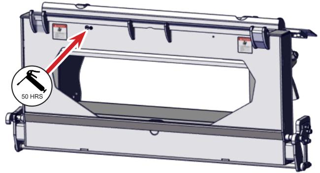
Slave Cylinder Barrell End and Pivot Pin
