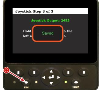
Push the Joystick lever all the way to the left and then press the Enter button (B).
