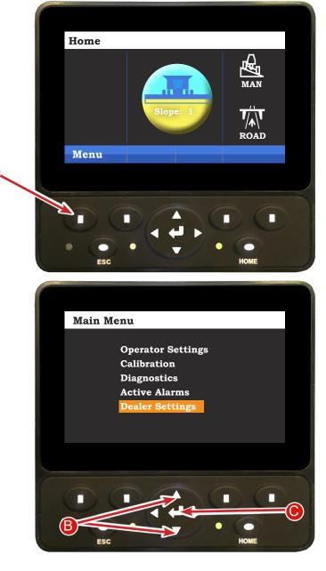
Push the up or down arrows (B) to move to the desired function. Once the desired function is highlighted press the Enter button ( $\checkmark$ ) (C) to go into that page. Press the Home button to go to the Home screen.
