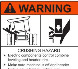
Make sure machine is off and header lock is down before making any adjustments to the electrical system.
