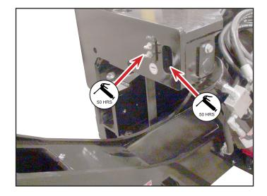
Master Cylinder (Base and Rod) 50 hrs. 2 Zerks
