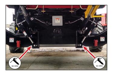
Leveling Cylinders Rod End 50 hrs. 2 Zerks
