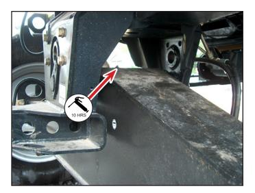
Steering Axle Pivot 10 hrs. 1 zerk
