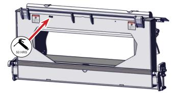
Slave Cylinder Rod End 1 zerk 50 hrs.
