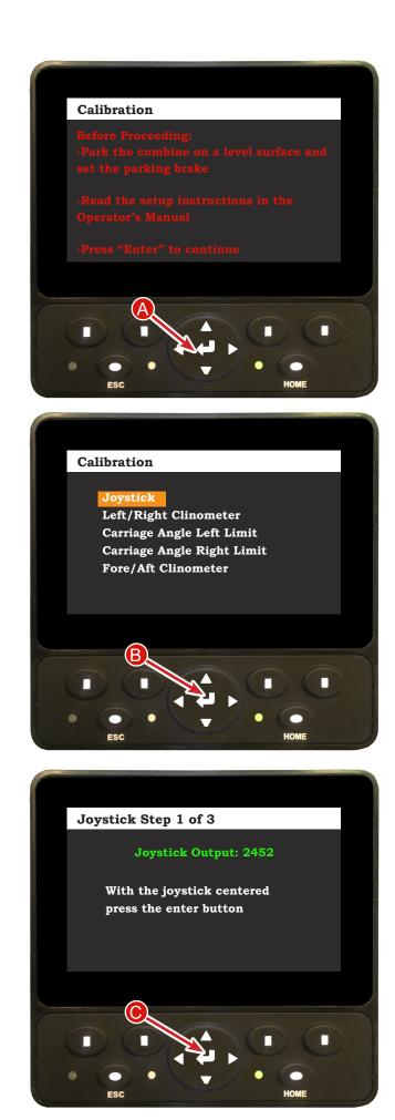
Push the Joystick lever all the way to the right and then press the Enter button (A).
