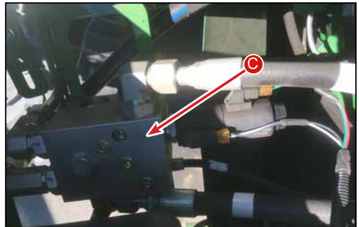
C - Leveling Manifold
