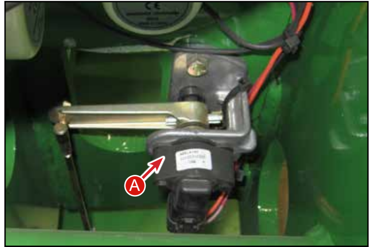
A - Overcarriage Position Sensor
