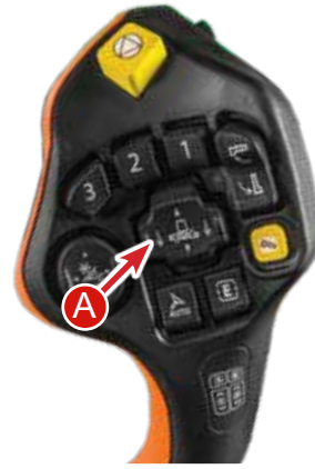
A - Header Trim Switch B - Master Cylinder
