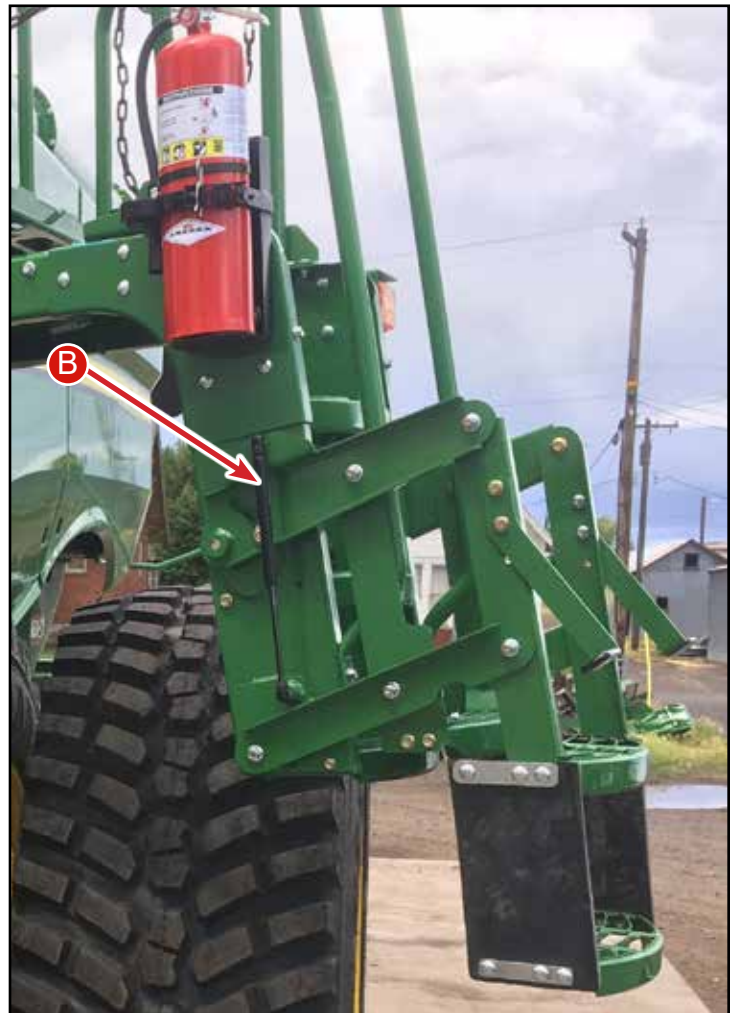
B - Gas-charged Struts
