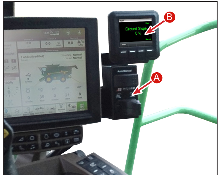
A - Leveling Control Switches B - Leveling System Monitor
