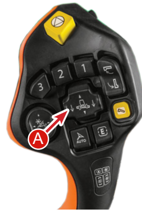
A - Header Trim Switch B - Master Cylinder
