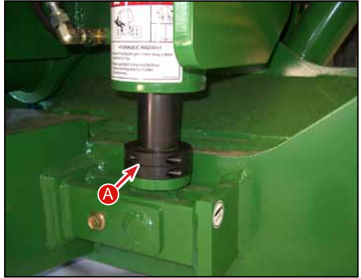
A - Mechanical Leveling Cylinder Stops 5/8 inch - Part # MC-137251 1/8 inch - Part # MC-137501
