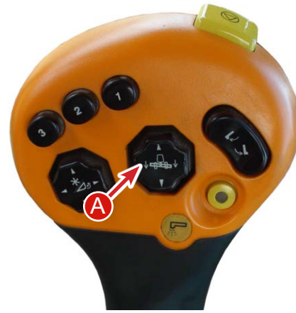
A - Header Trim Switch B - Master Cylinder
