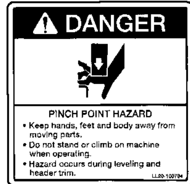
Label #3 Part number: LL20-10784 Locations: 2 (left and right side of upper transition face plate)
