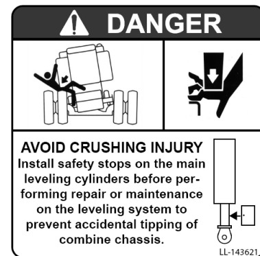
Label #9 Part number: LL-143621 Locations: 2 (Front of under carriage)
