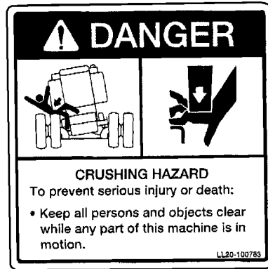
Label #2 Part Number: LL20-100783 Locations: 4 (Rear of undercarriage, and above rear axle)
