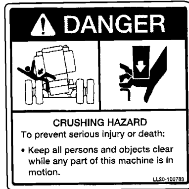
Label #2 Part Number: LL20-100783 Locations: 6 (front of undercarriage arms, frame mount area, and each rear side of combine)
