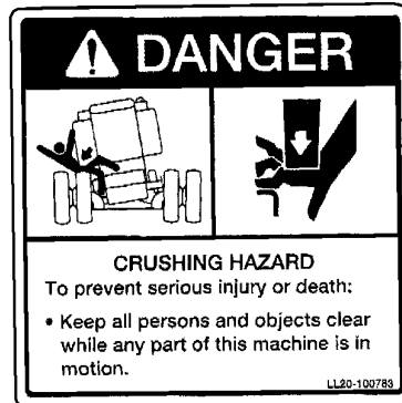
Label #2 Part number: LL20-100783 Locations: 6 (front and back of quarter circles and each rear side of combine)
