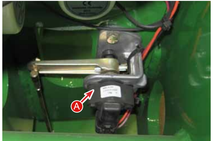
A - Undercarriage Position Indicator
